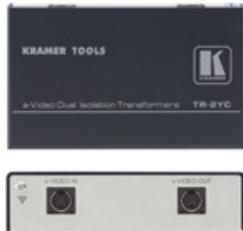
The TR-2YC is a high-performance isolation transformer for s-Video (Y/C) signals. It provides complete isolation between devices to eliminate hum, ground loops and DC offsets, which can degrade the video quality
